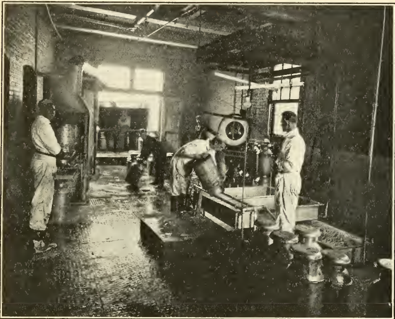
FIGURE 2.—Receiving milk at a plant using system 3. An average of 289.9 gallons per man-hour and 1,079.6 gallons per hour was received at 20 plants using this system
